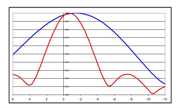
If you are currently using a 12 bay batwing, going with a lower gain **TPV-SFN** antenna will greatly enhance reception in urban and hilly areas. The lower gain **TPV-SFN** will provide up to 70% more field at low depression angles. This will greatly help with building penetration. As we have said before, adding elliptical polarization is just icing on the cake in helping to get your signal to viewers.
