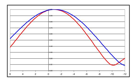
The beam tilt of both antennas on the upper plot is 1.0 degree. In the lower plot we have changed the beam tilt of the TPV-SFN 5 bay antenna to 1.5 degrees. The gain of the antenna did drop slightly to 5.80, (or 7.63 dB). Note the field values are up to 30% higher at some depression angles, compared to the standard 6 bay antenna.
