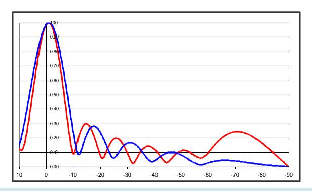
The elevation gain of the **TPV** antenna is 6.00, (7.78 dB), while the 5 bay **TPV-SFN** antenna has a gain of 5.95, (7.74 dB). Since the **TPV-SFN** has greatly reduced high angle grazing lobes (in this case, around +/- 70 degrees), the aperture efficiency of the array increases substantially.
