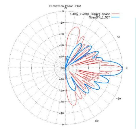
Here is a polar plot of the 12 bay batwing (RED) and the 5 bay TPV-SFN antenna with 1.5 degrees of beam tilt. Even with the 12 bay antenna there is a lot of signal wasted in the two high angle grazing lobes. These lobes do nothing more than fire more RF into the ground near the tower, and also wastefully up into space.
