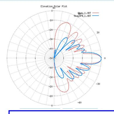
To the left is the same set of elevation patterns shown in polar form. The TPV-SFN antenna, (Blue), produces much higher radiation at lower depression angles hence the higher elevation gain and up to a 25 dB reduction in RFR hitting the ground.
